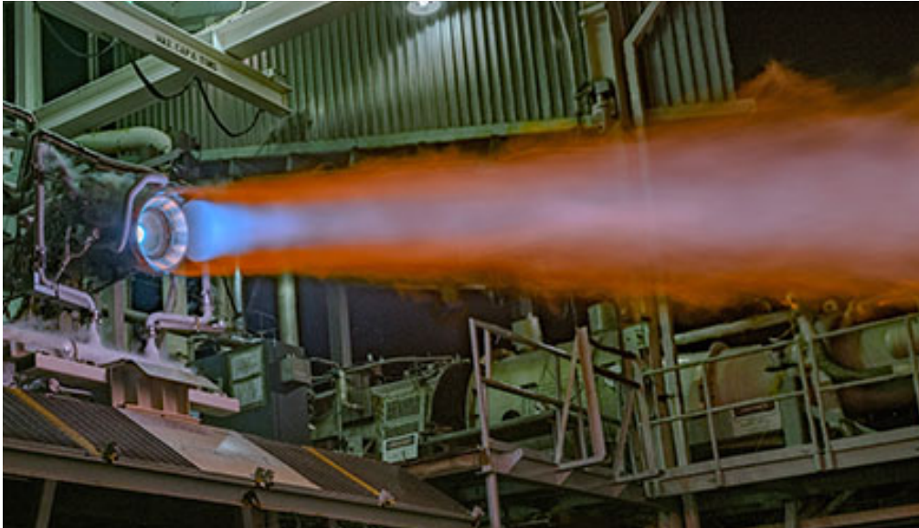
Below: Reaction Control Thruster for Orion Spacecraft Crew Module
